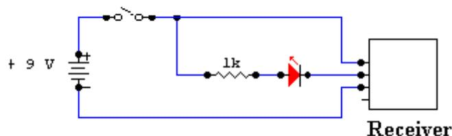
This circuit causes the LED to light for every heart beat and/or transient detected: in this way it is possible to determine whether there is electromagnetic noise, and identify its source.
