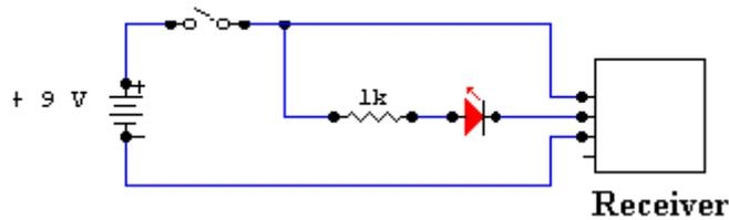
The circuit lights the LED for every heart beat and/or disturbance that is received: in this way it is possible to determine whether there is any interference, and identify its sources.
